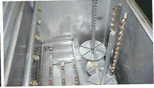
The ultrasonic washing units series U 650 are engineered for the narrow web printing industries (labels). This washing unit allows easy and economical cleaning for the cylinders and sleeves. The ink left in the cylinders or sleeves during the printing process is removed thanks to the mechanical action caused by the ultrasonic cavitation in a solution of water and detergent.
